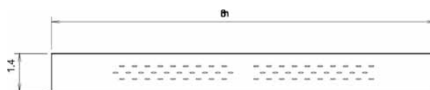
Fig. 8.b: Schematic transversal cross-section of the LTCC based reactor through three layers of buried channels on the right (reformer) part of the structure.
