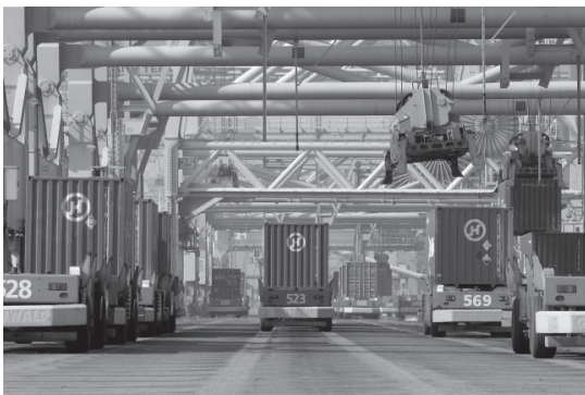
Fig. 2. Autonomous AGV's (automated guided vehicles) in the Rotterdam Port ECT sea container yard, operational for almost two decades now [source: www.ECT.nl].
