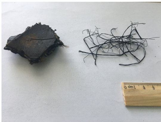
Fig. 3 Waste tyres components: left – rubber; right – steel (Authors own processing)
