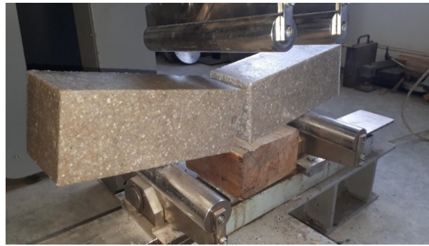
Fig. 8 Load layout scheme
