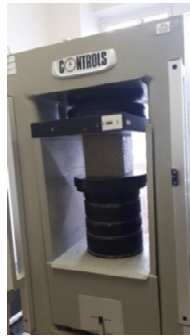
Fig. 3 Compressive strength testing
