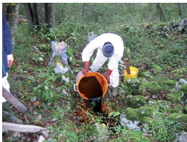
Fig. 5. A solution of uranium was injected into a well permeable fissure at the margin of the landfill.
