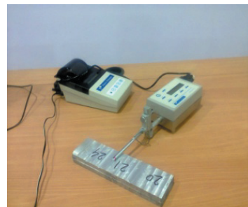
Fig. 2. Surface roughness measurement using Surtronic 3+
