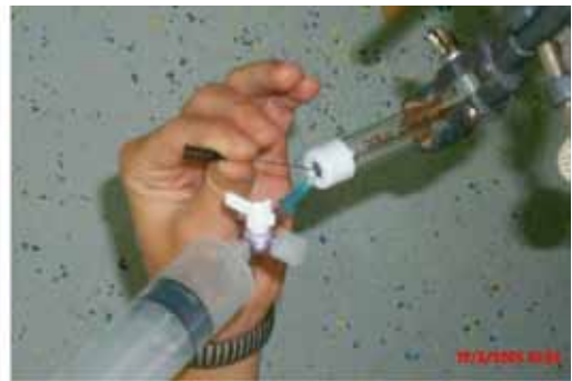
Figures 4. (left) and 5. (right): Gas sampling into a piston ampoule (1 bar) from autoclave (at 60 bar to 100 bar), and then transferring of gas to a laboratory ampoule.
