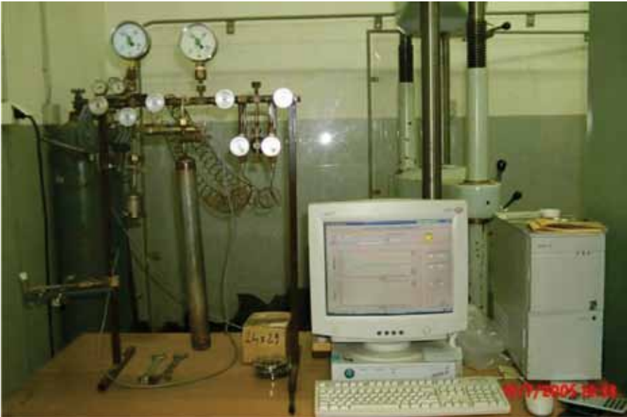
Figure 1. Modernized apparatus for sorption measurements - autoclave, probe, valves, software application
