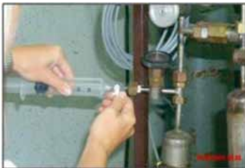
Figures 4. (left) and 5. (right): Gas sampling into a piston ampoule (1 bar) from autoclave (at 60 bar to 100 bar), and then transferring of gas to a laboratory ampoule.
