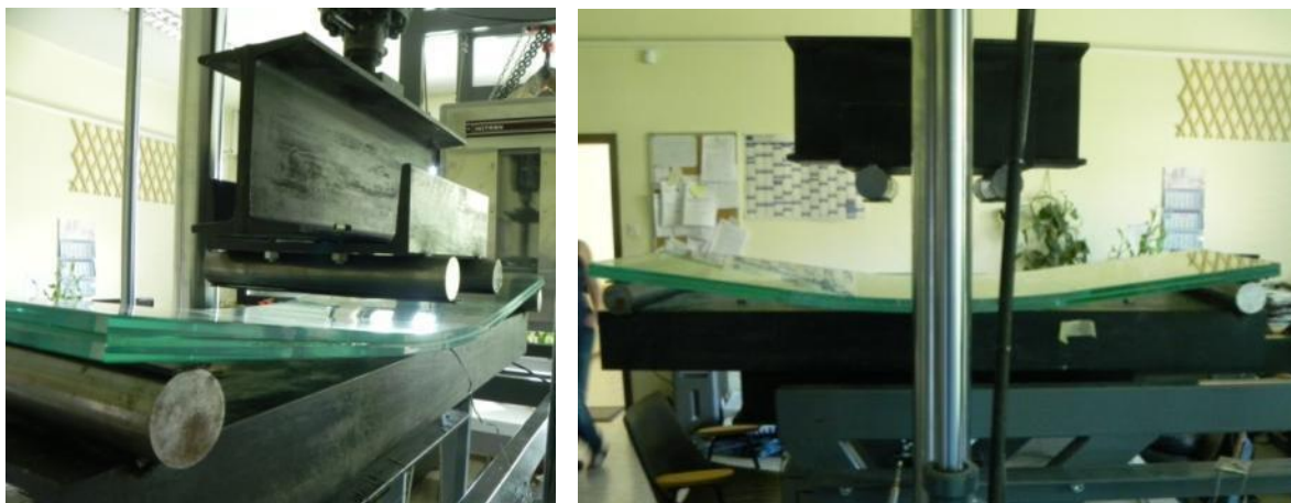
Slika 22: Preizkušavec po poružitvi obeh steklenih lamel. Figure 22: Specimen after the failure of both glass laminas.
