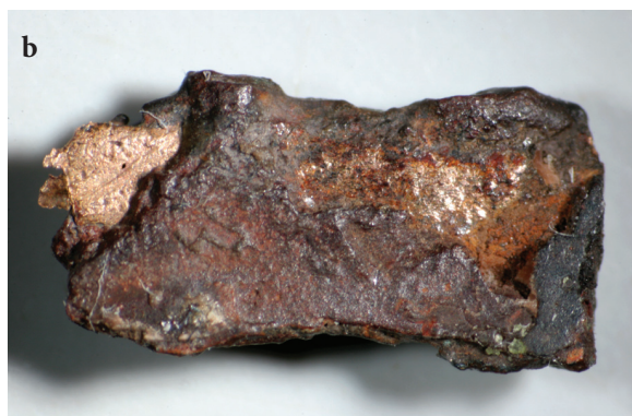
Fig. 4: Fragment of the 3 rd front bridge (0.9 cm long). a: top – chalcopyrite on the surface of the fragment and a layer of bronze on the left; b: underside – two layers of bronze. Not to scale (photo: S. Perovšek).
