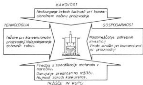
Slika 7 Razlogi za uporabo EPŽ postopka 3 Fig. 7 Reasons for the application of the ESR process 3
