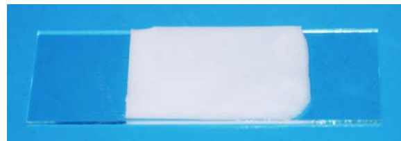
Figure 8.2: Prepared agar layer with scatterers ( \text{TiO}_2 ) on a microscope glass slide.
