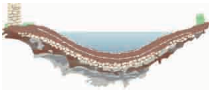
Slika 8: At other locations, clay was tamped down firmly on the bottom; this method required more careful maintenance of the water hole, in order to prevent leakages (sketch 3).
