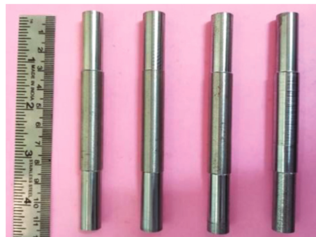
Figure 1: A few samples of turned P235GH steel rods
