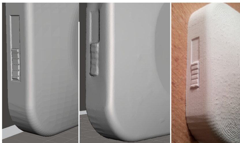
Fig. 5 Detail of original (left), scanned (middle) and printed (right) front camera cover
