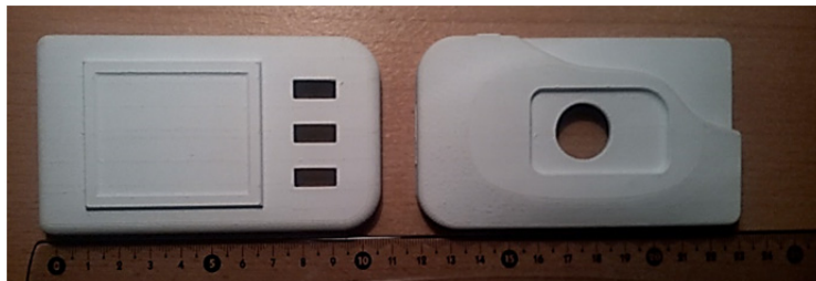
Fig. 2 3D printed models of camera casing
