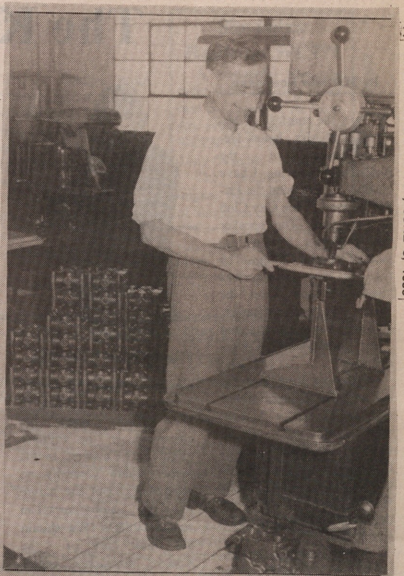
That's me at the tapping machine. The machine cuts threads inside a drilled hole. Behind me are the steel parts that need tapping.
