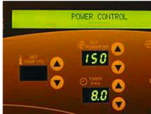
Figure 1. Radiofrequency generator with multiple temperature displays and impedance and power monitoring.
