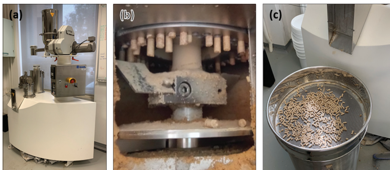
Slika 2. Laboratorijska peletirna naprava Kahl 14-175 (a), proizvodnja peletov (b) in ohlajevanje peletov (c). Figure 2. Laboratory pellet press Kahl 14-175 (a), pellet production (b) and cooling of the pellets (c).
