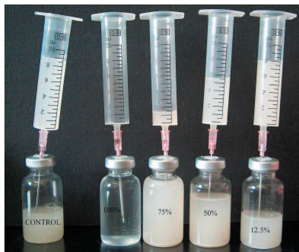
Figure 2. Yeast toxicity test – gas production in control bottle and in bottles with different dilutions (100, 75, 50, 12.5%) of original wastewater.
