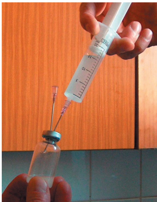
Figure 1. Broth bottle syringe yeast toxicity test – sample inoculation employing two needles.
