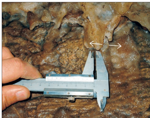
Fig. 3: An example of the speleothem damage measured along the main corridor of the cave. The arrows on the photograph indicate the direction of displacement (Photo: M. Briestenský).
