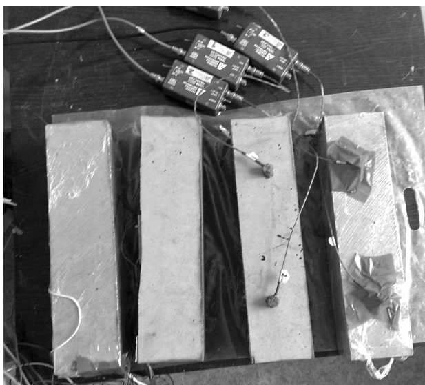
Figure 2: Experimental set-up after unmoulding (sample S1 and S4 are covered, S2 and S3 are uncovered)
