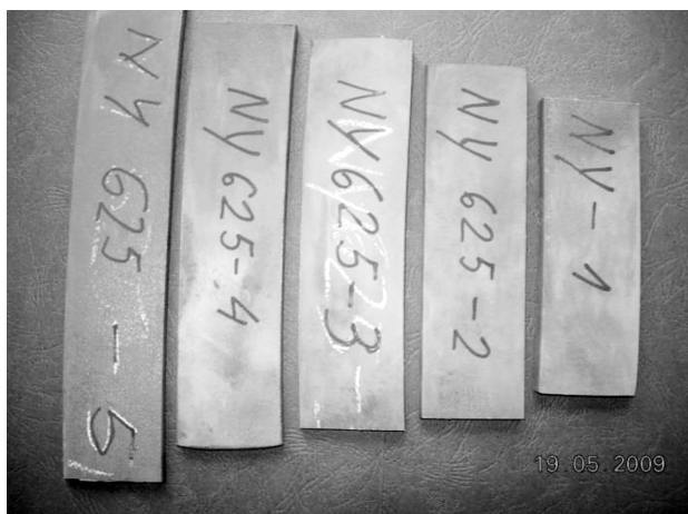
Figure 1: Hot rolled and air cooled specimens of Inconel 625, subjected to different numbers of rolling passes
