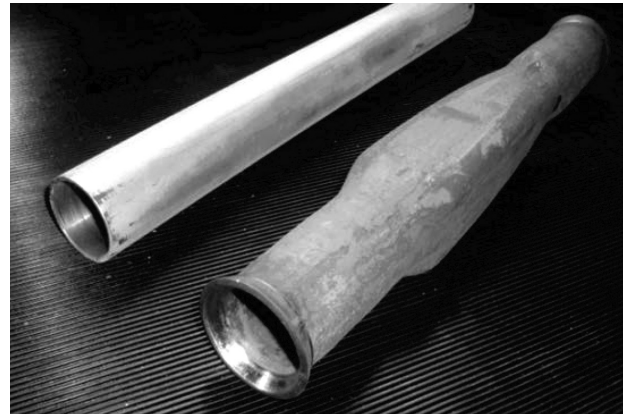
Figure 2: Experimental stock and the resulting shape after hot stamping
