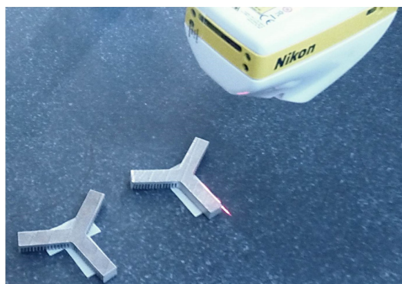
Fig. 6. Part measurement with a non-contact laser scanner
