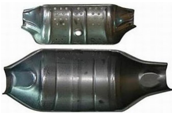
Fig. 1. Schematic diagram of automotive catalytic converter
