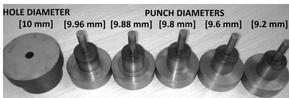
Fig. 6. One set of manufactured punches ( t/D_m=1/5 )
